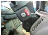
Engine stop through the key close to the steering wheel inside the cab.
