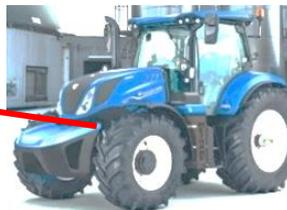
Using ignition key or rod push the button to unlock whilst lifting the hood with two hands.
